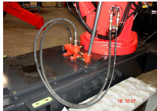
Illustration 5 showing crane ready for emergency winching
